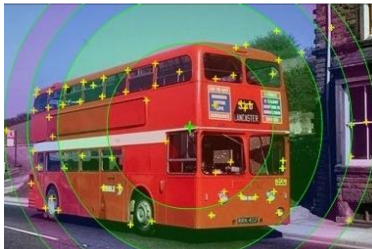
Figure 3.3 The set of SDPF points allocated to the set of distance bins. The yellow markers show the SDPF points, whereas the green cross marker is the centroid. The coloured bands are the distance bins.
