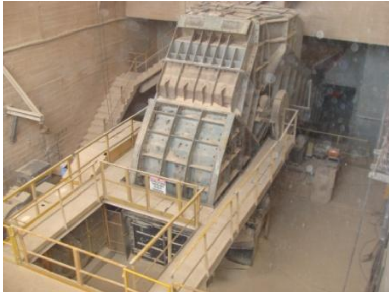
Figure 2-7: Hammer type raw material crusher at HLL - PCW
