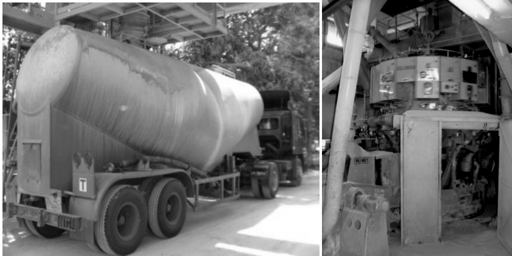
Figure 2-19: Dispatching: bulk tankers for industrial use (L), packer (R)
