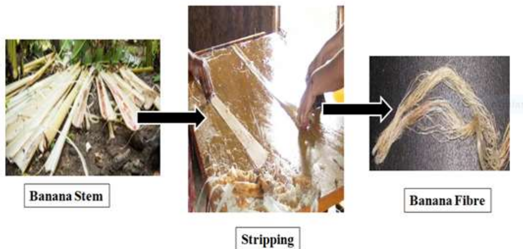
Figure 2-16 Banana fibre stripping process steps
