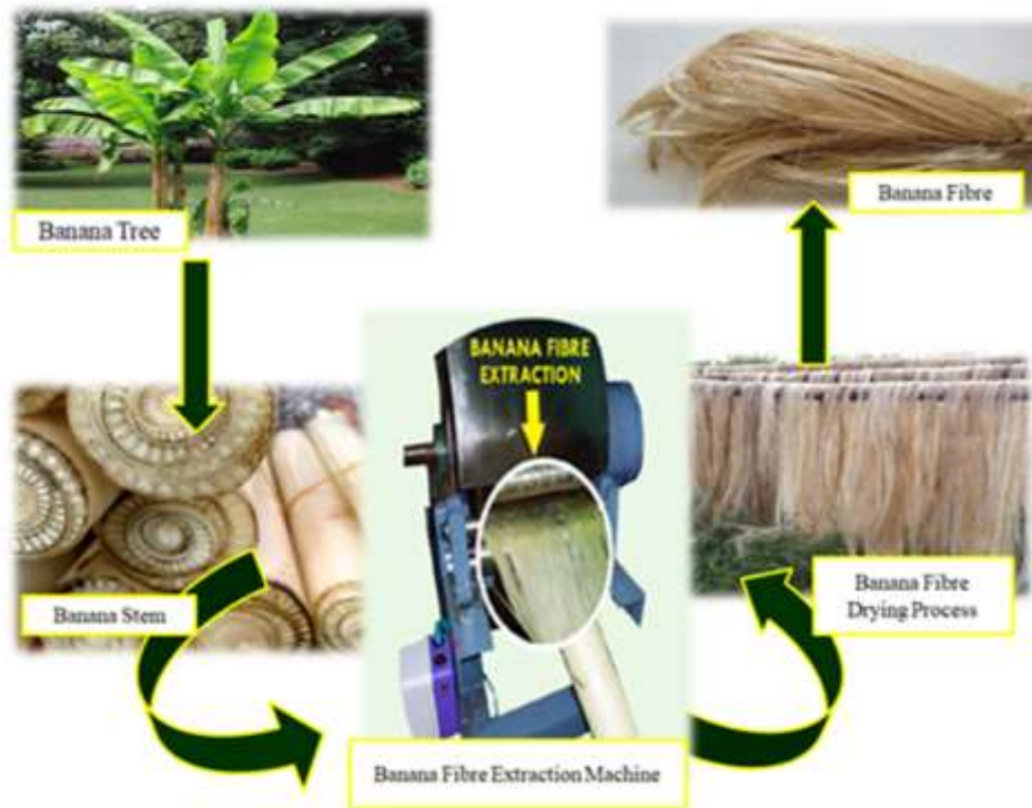
Figure 2 14- Banana fibre extraction process
