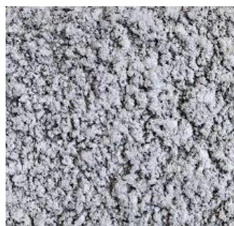
Figure 30 : Grade 15 Chip concrete (1:2:4)
