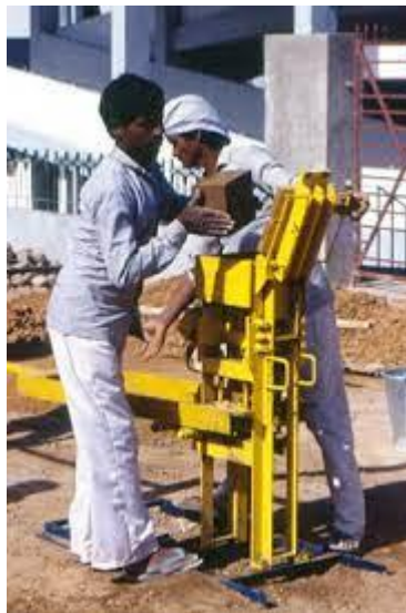
Figure 9: Hand pressed block manufacturing
