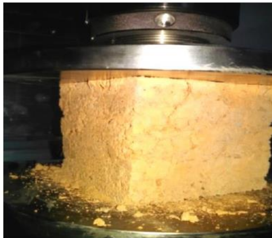
Figure 8: Compressive strength testing for CSEB
