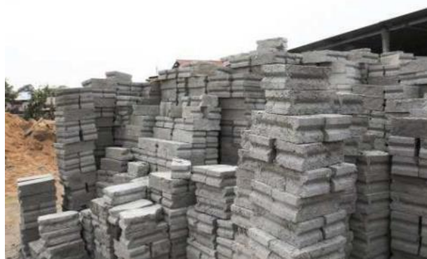
Figure 1 : Cement Sand Block (CSB)
