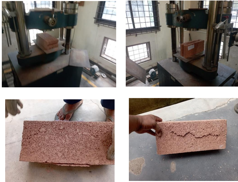
Figure 29 : Performance of compressive strength test
