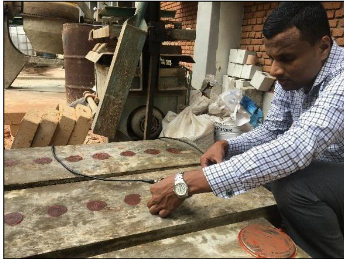
Figure 3.8 (b); Testing for UPV Measurements on Test Panels in Series 2
