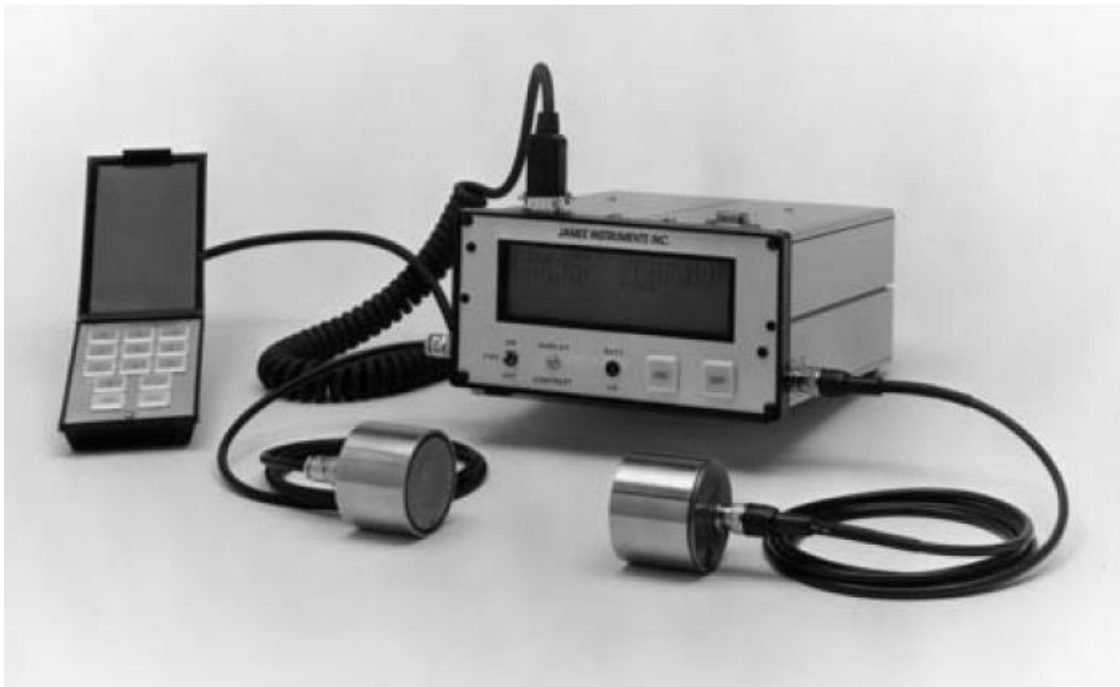
Figure 3.2; Typical UPV Testing Instrument (Tarun et al., 2004)
