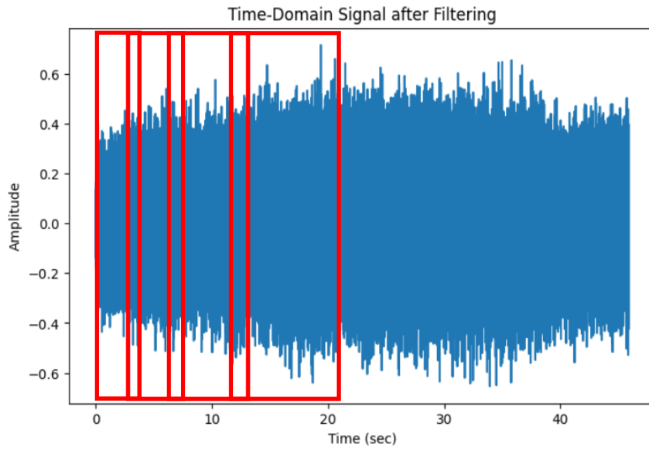
Figure 2.10: Adaptive Windowing & Window shifting in Time Domain
