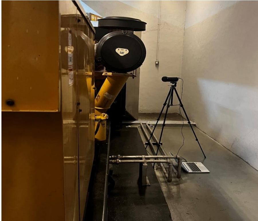
Figure 3.6: Apparatus for collecting audio signals from the generator
