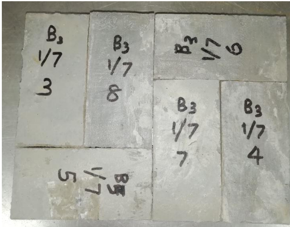
Figure 4-5 Delamination of type 03 paving Block
