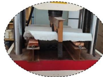
Transverse Strength Test on MCR Tiles (Accordance with SLS 1189: Part 1 and 2)
