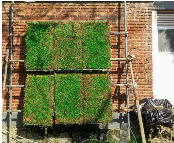
Figure 6.12: Experimental setup of the vertical modular panel green wall system
