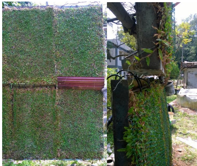
Figure 6.11: Measuring the water requirement of a single panel
