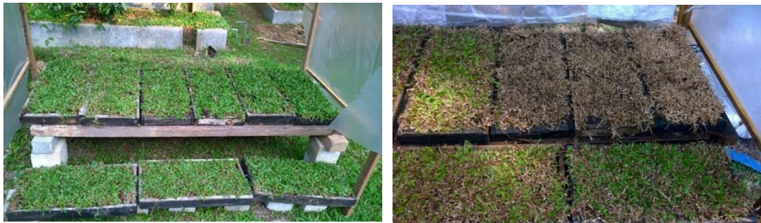
Figure 6.10: Field tests conducted for permanent wilting point investigation
