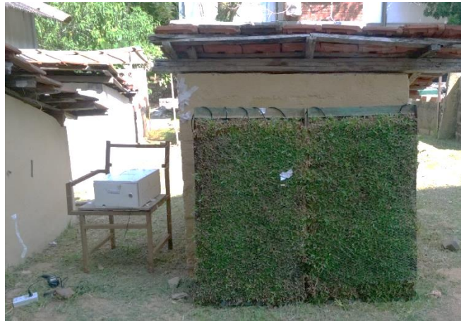
Figure 6.5: Thermal performance analysis of the panels
