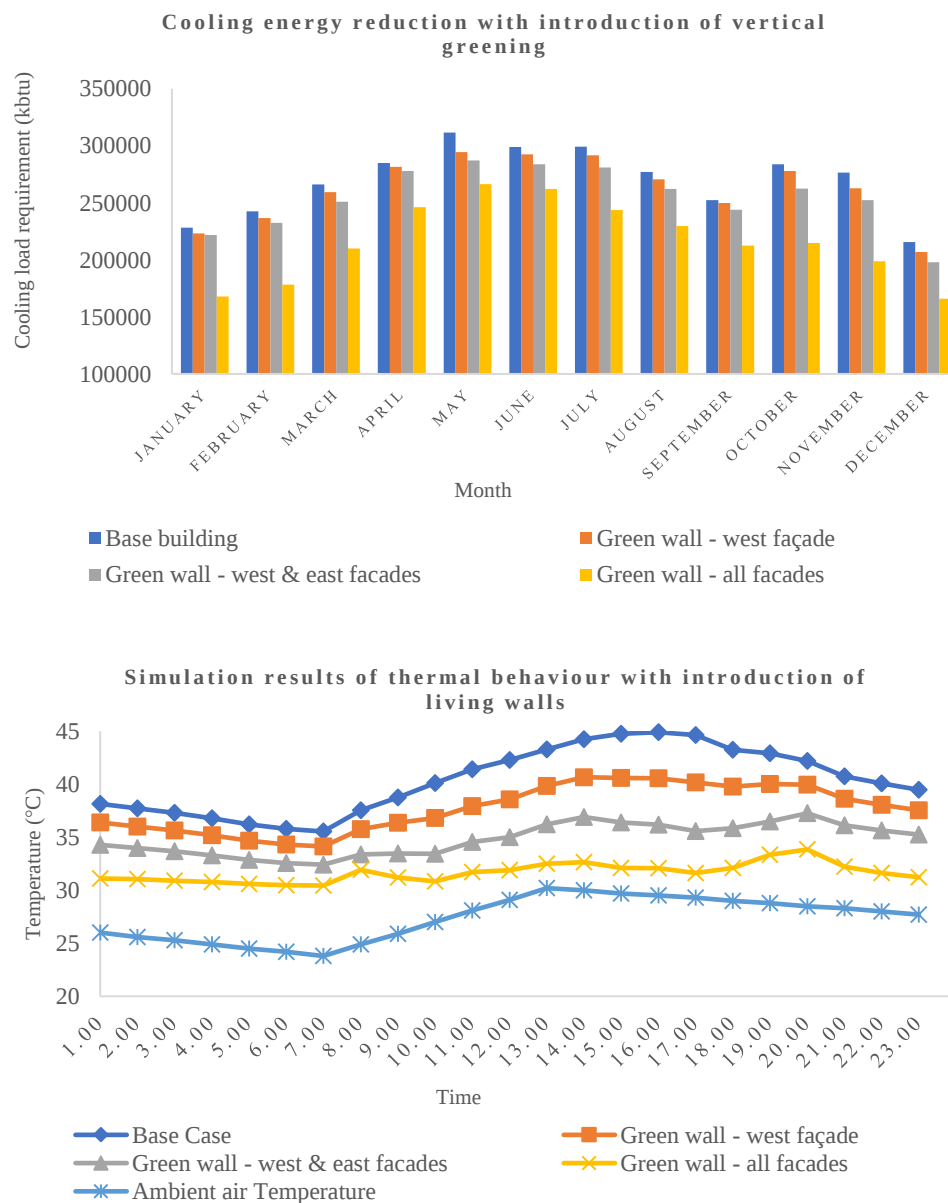
Figure 7.2: Results of the pilot study in building scale
