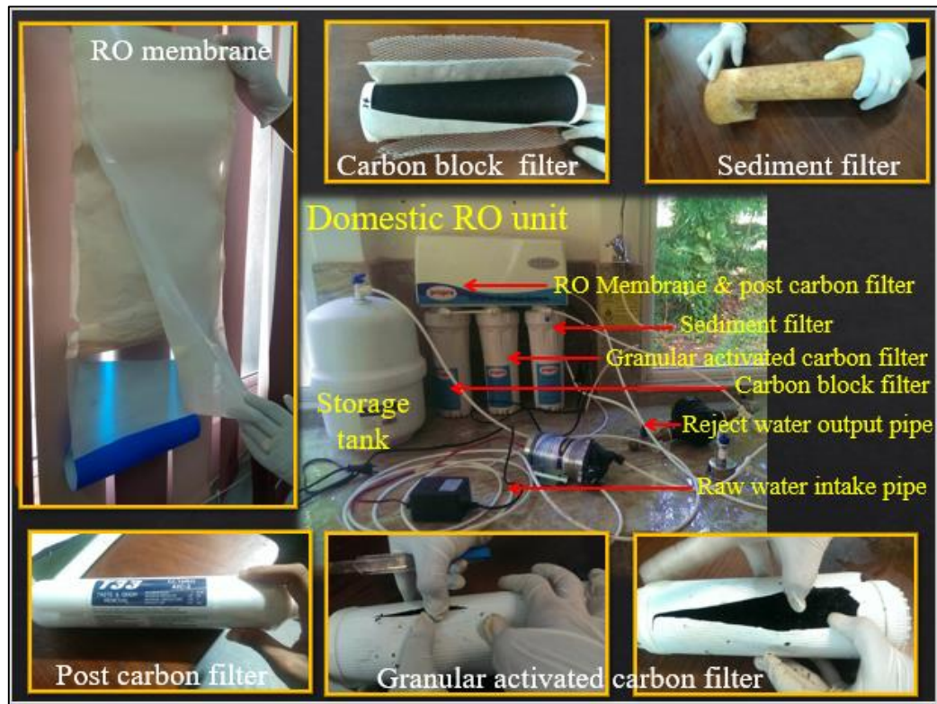
Figure 2.2: Different components in the RO filter unit
