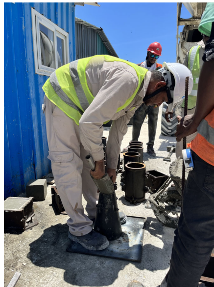
Figure 3.11 : Preparation for the slump test
