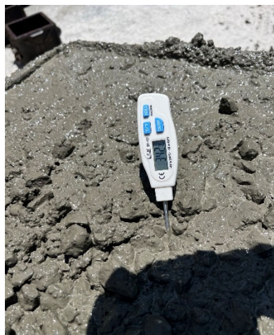
Figure 3.10 : Temperature reading on the fresh concrete in day 1
