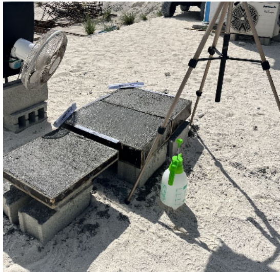
Figure 3.13 : Test setup for the monitoring of shrinkage cracks
