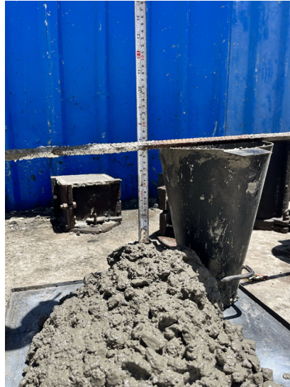
Figure 3.12 : Slump measurement of the fresh concrete in day 1
