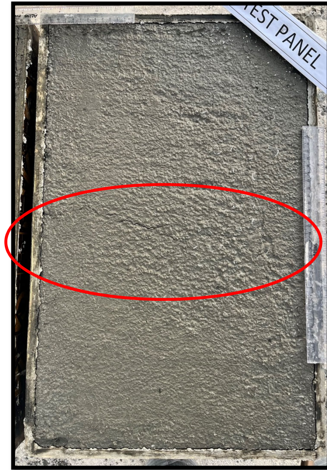
Figure 4.8: Crack pattern of the concrete mix of fresh concrete temp. 32.7 °C
