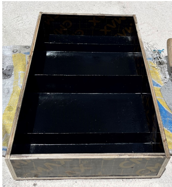
Figure 3.6 : 3D view for the mould for the measurement of plastic shrinkage cracks
