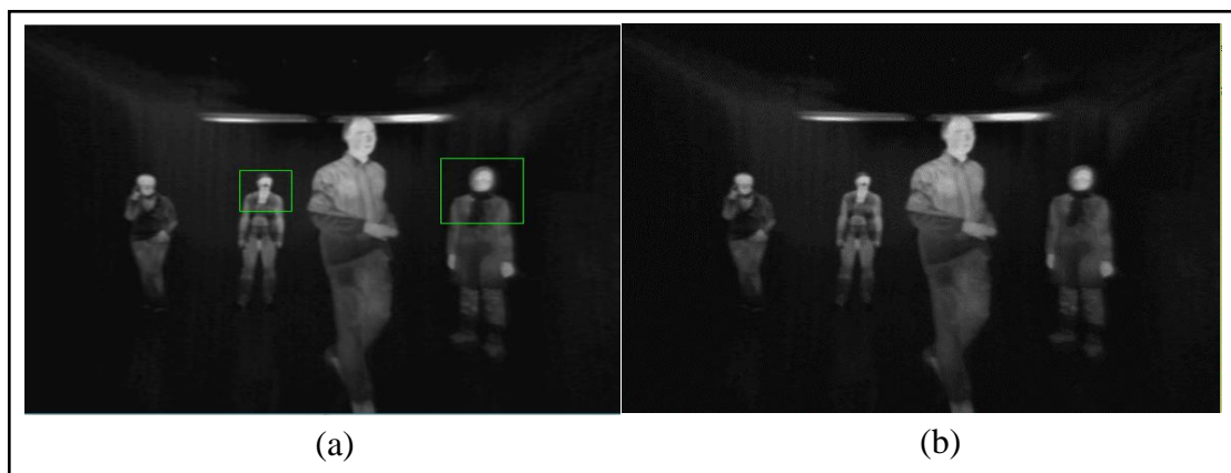
Figure 11: Human detection using (a) haarcascade_mcs_upperbody.xml (b) haarcascade_fullbody.xml classifiers
