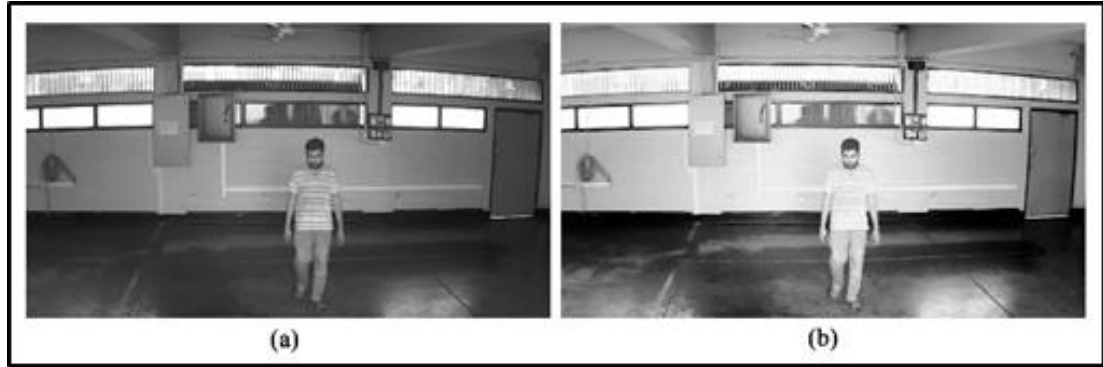
Figure 20: The preprocessing using histogram equalization (a) raw image (b) enhanced image after histogram equalization
