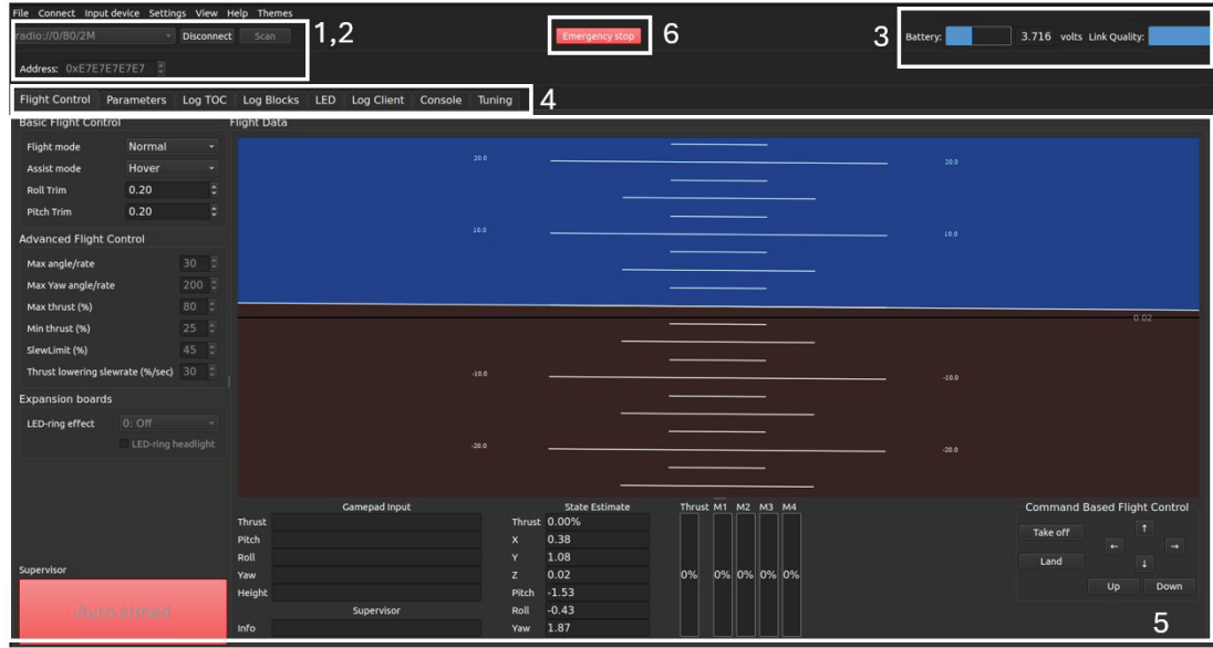
Fig. 3.2: User interface of CFClient for connecting to, controlling, and logging data from the Crazyflie.
