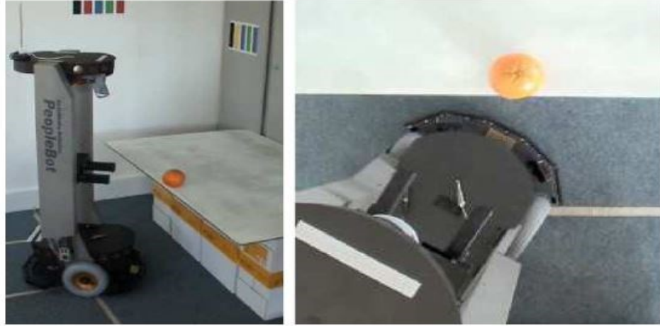
Figure 2.7 Mobile robot docking behavior to grasp the orange fruit
