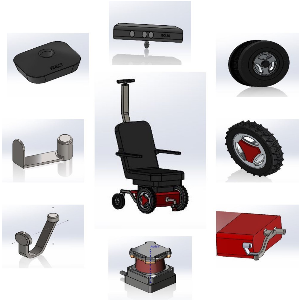
Figure 3.6 Solid work design of the wheelchair
