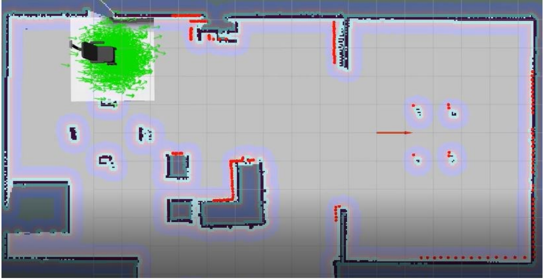
Figure 4.4 Wheelchair initial pose array indicates in green color and goal posed indicates in red arrow.
