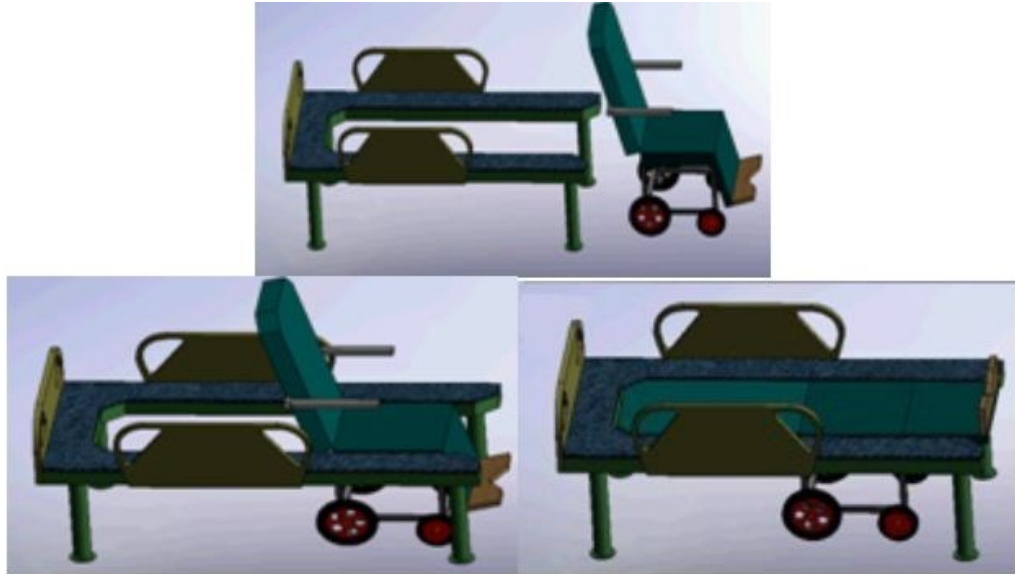
Figure 2.3 wheelchair's docking process in U shaped bed
