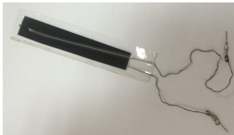
Fig. 2.5 Approach with Velostat and conductive yarn
