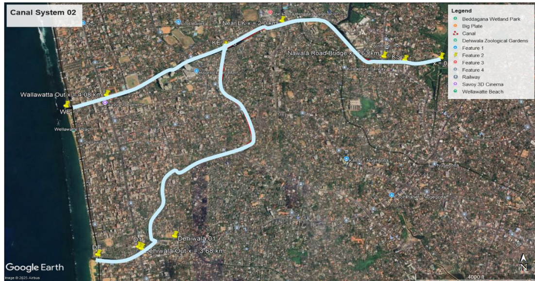
Figure 49: Dehiwala-Wellawatta-Kirillapone Canal System, showing four water level monitoring stations, Nawala Road Bridge (0.63 km), near Lanka Hospital (2.00 km), Wellawatta Canal Outlet (4.08 km) from the canal origin (x = 0 m) in the Kirillapone Canal, and Dehiwala Canal Outlet (3.68 km) from the connection junction
