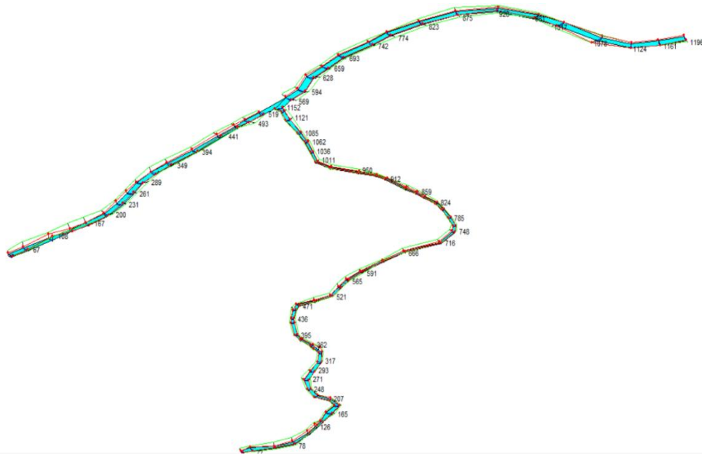
Figure 59: Maximum flood condition along the Dehiwala-Wellawatta-Kirulapone canal system on 10/14/2025
