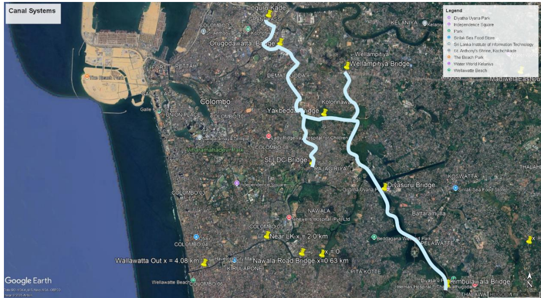
Figure 65: Parliament Lake-Kiththampahuwa-Kinda-Dematagoda Canal System, showing four water level monitoring stations, Kimbulawala Bridge at the canal origin ( x = 0 m), Diyatha Bridge (3.780 km), Yakbedda Bridge (7.530 km), Orugodawatta (10.900 km), and Ingurukade Junction (12.100 km)
