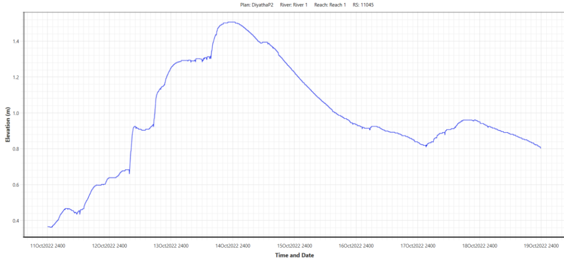
Figure 72: Stage hydrograph at Kimbulawala Bridge water level station used as the upstream boundary condition for Canal System 3
