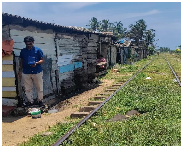
Figure 1.2: Vibration measurement at the Koralawella site
