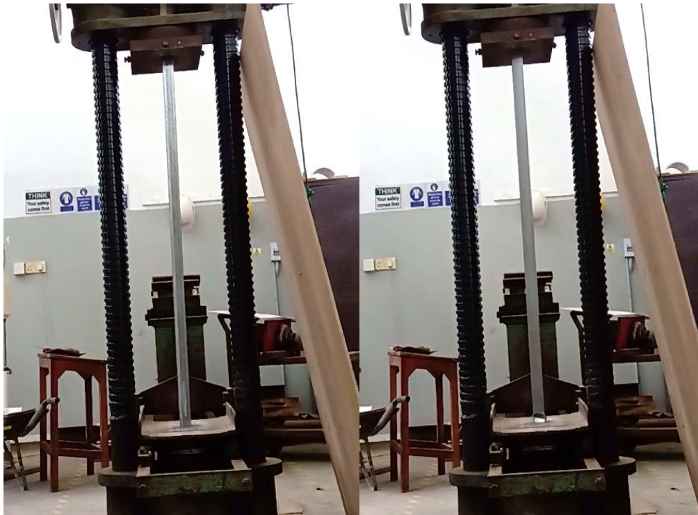
Figure 4.1: Compressive load test of hollow GI section (1.5 m high, 1.2 mm thick)
