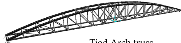
Tied Arch truss
