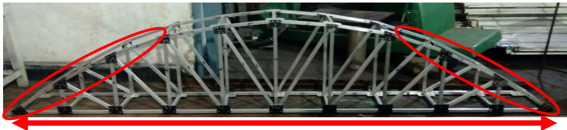
Figure 5.12: Concrete grout infilled members in truss B
