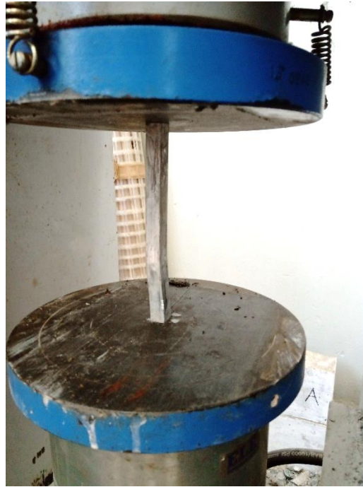
Figure 5.7: Testing of individual members of model trusses
