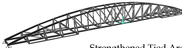
Strengthened Tied Arch truss
