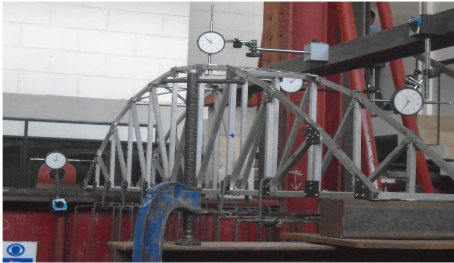
Figure 5.18: Dial gauge setup
