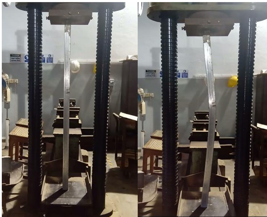
Figure 4.1: Compressive load test of hollow GI section (1.5 m high, 1.2 mm thick)
