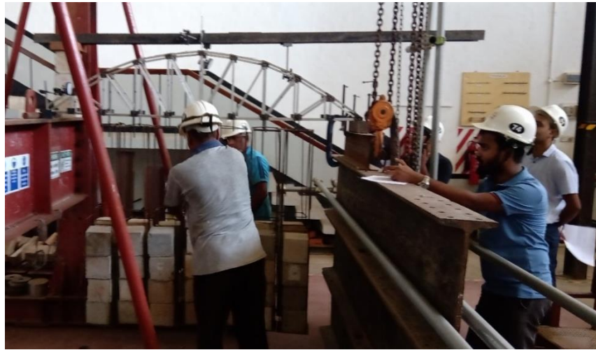
Figure 5.17: Loading of truss bridge in the laboratory
