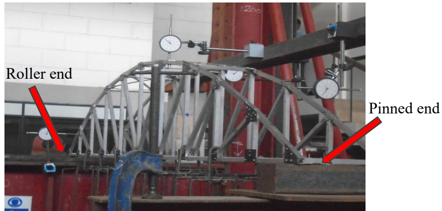
Figure 5.15: Support conditions of tested trusses
