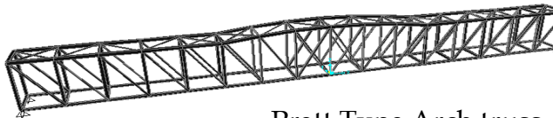
Pratt Type Arch truss
