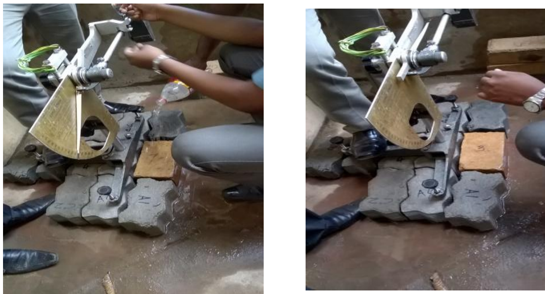
Figure 36 : Skid resistance testing process
