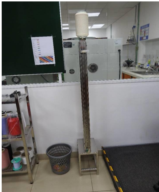
Figure 2-3: Customized setup to measure unevenness
