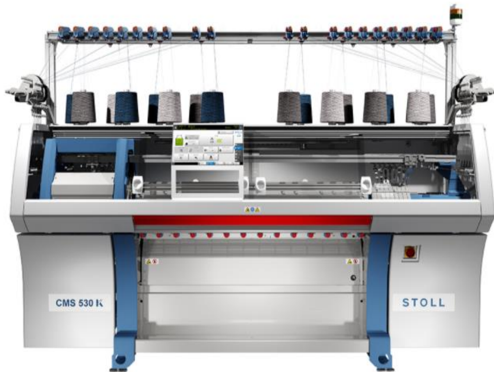
Figure 3-11: Stoll HP 530 Flat knit machine
