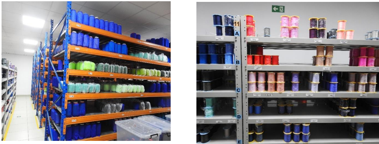
Figure 5-5: Yarn Storage Racking
