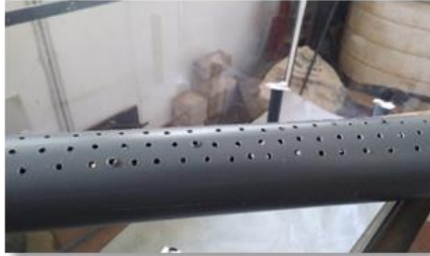
Figure 3.15: Perforated PVC pipe used as a drain
