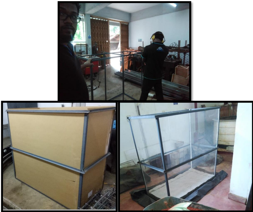
Figure 3.2: Construction of box for laboratory model with steel frame and acrylic sheet walls on all four sides
