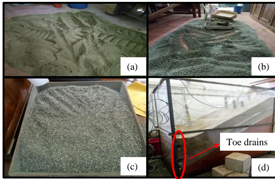
Figure 3.21: Construction stages, (a) air drying the river sand, (b) air drying the M-sand, (c) air dried M-sand sample ready for filling, (d) Fully constructed and instrumented 30° slope model
