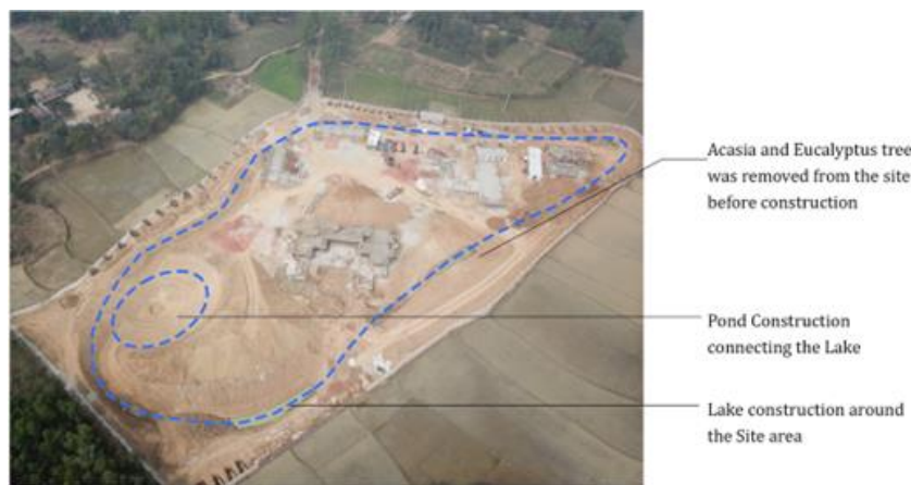
Figure 5 Creating a lake surrounding the site to regenerate the historic landscape formation
