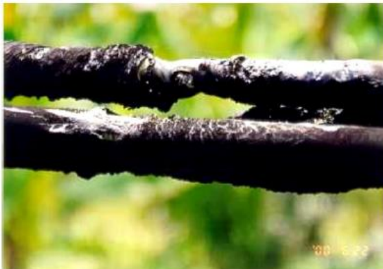
Figure 11 : Outer sheath damage of MVABC
