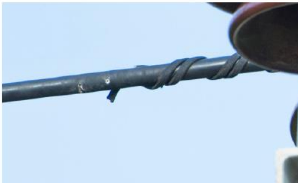
Figure 14: Cable insulation damage from use of metallic dead-end clamp.
