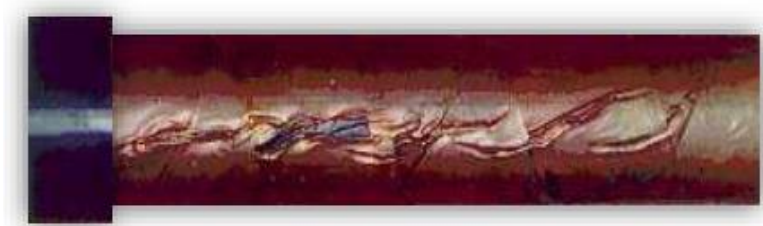
Figure 11 : Outer sheath damage of MVABC
