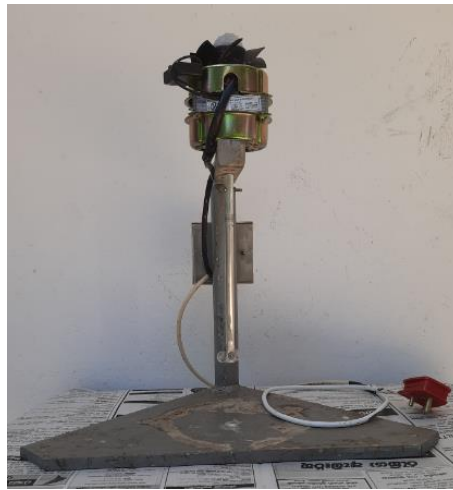
Figure 3.6: internally fabricated mixing unit used for coating mixing
