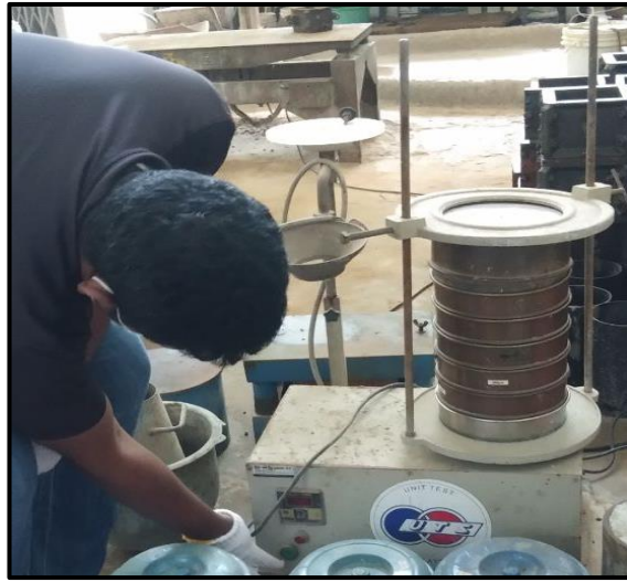
Figure 26: Sieve shaker used for the sieve analysis
