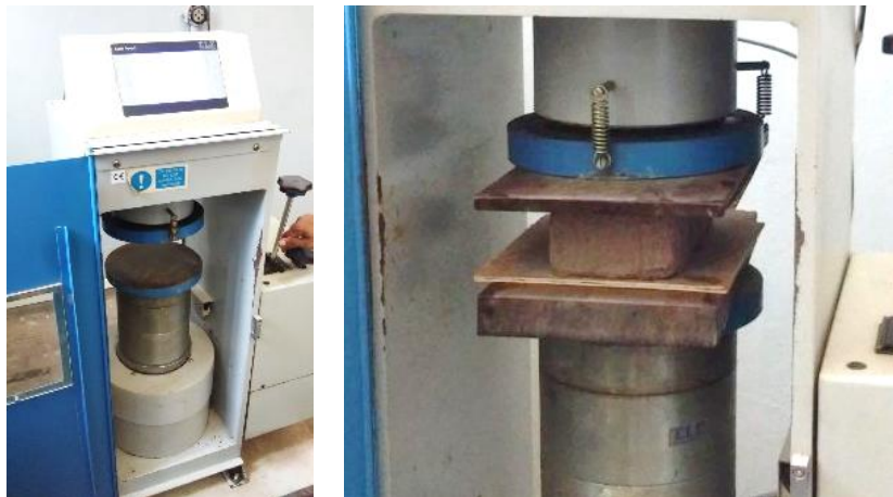
Figure 39: Machine used for compression test on blocks
