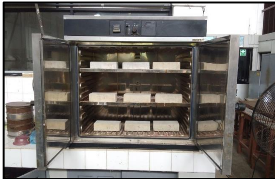
Figure 43: Oven used to conduct the water absorption of the paving alternatives
