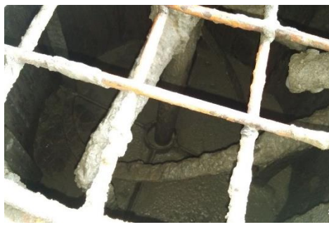
Figure 10: Picture of the inside of the aircrete mixing equipment
