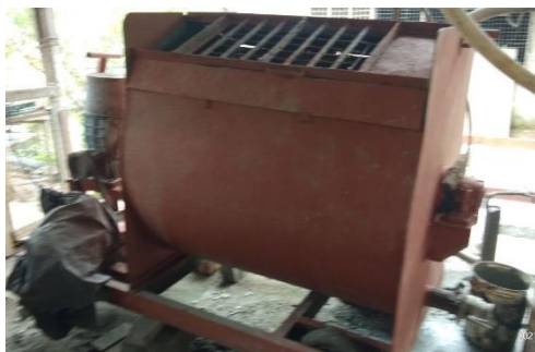
Figure 9: Aircrete mixing equipment
