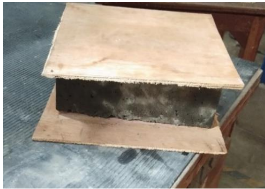
Figure 38: 4mm plywood packing provided at the time of testing
