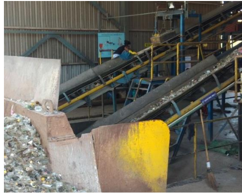
Figure 14: Used glass products fed to the washing drum
