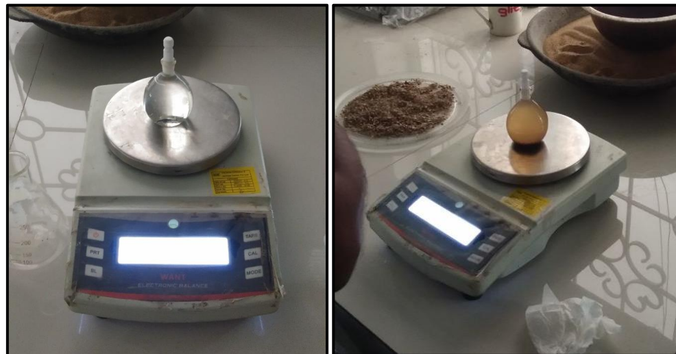
Figure 28: Pycnometer measurements obtained during the SSD specific gravity calculation
