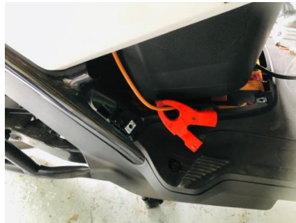
Fig. 3.2: Attachment of clip-on meter clip to the main power line.
