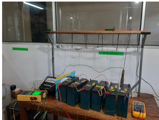
Fig. 3.3: Laboratory experimental set up for Lead acid battery testing.
