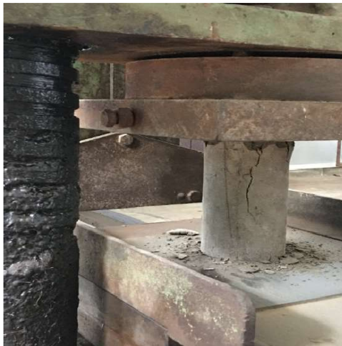
Figure 3. 18: Unconfined compression experiment on a sample prepared
