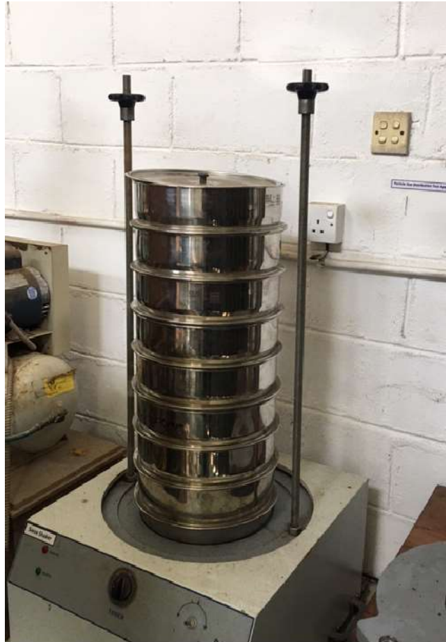
Figure 3. 11: Sieve analysis apparatus setup
