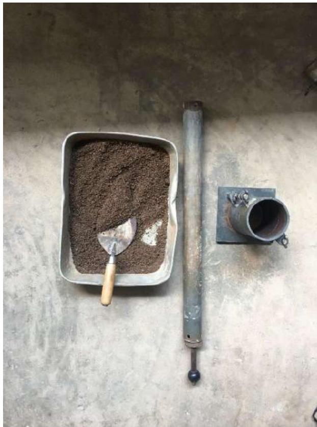
Figure 3. 13: Modified proctor hammer and mold
