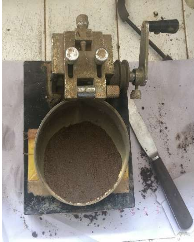
Figure 3. 12: Atterberg limit apparatus setup
