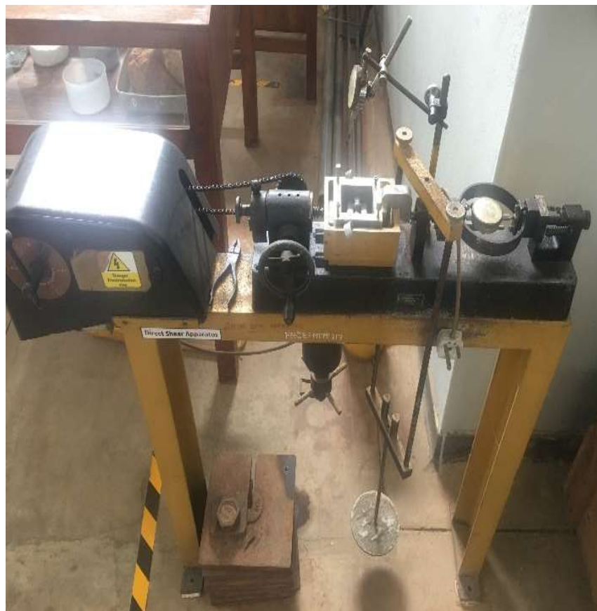
Figure 3. 14: Direct shear apparatus
