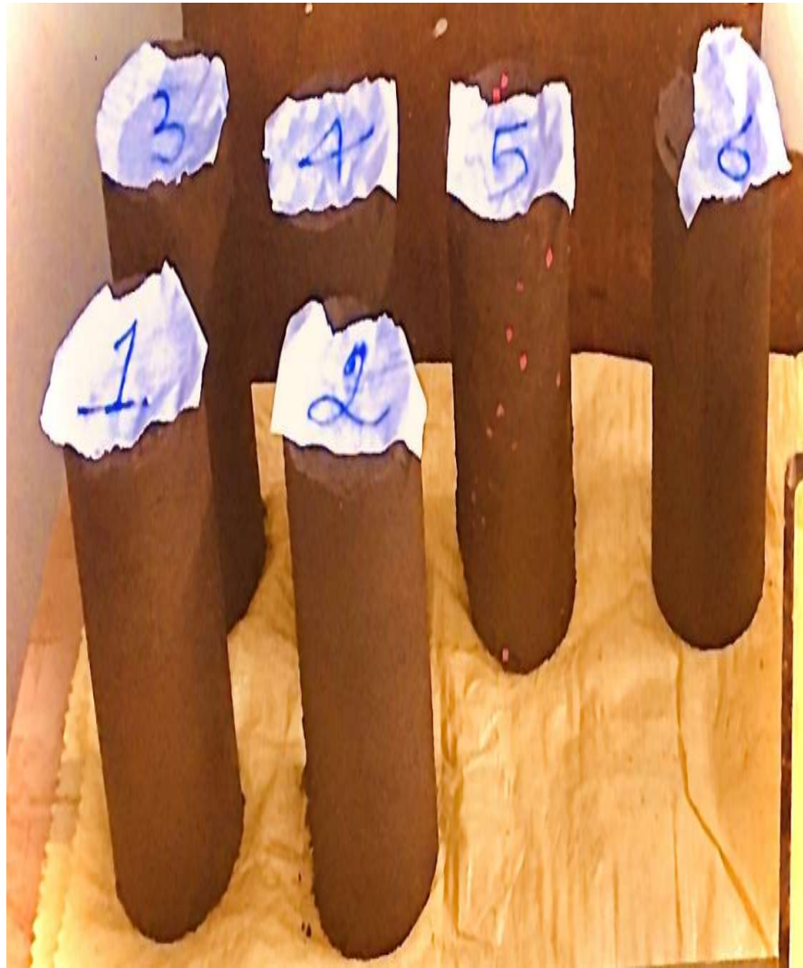
Figure 3. 16: Samples prepared for unconfined compression test
