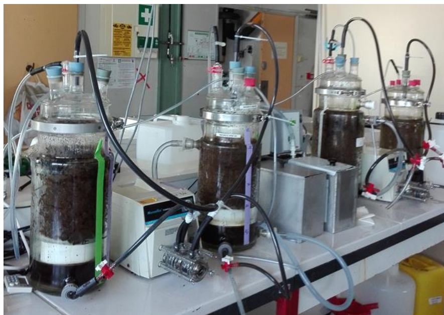
Figure 9. Leach bed batch reactors Setup
