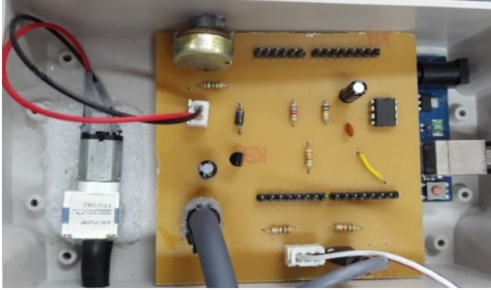
Fig. 3.5: PCB designed for PAT signal Data acquisition
