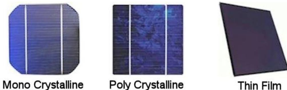
Figure 2.17: Different Type Solar Cells Construction Appearance
