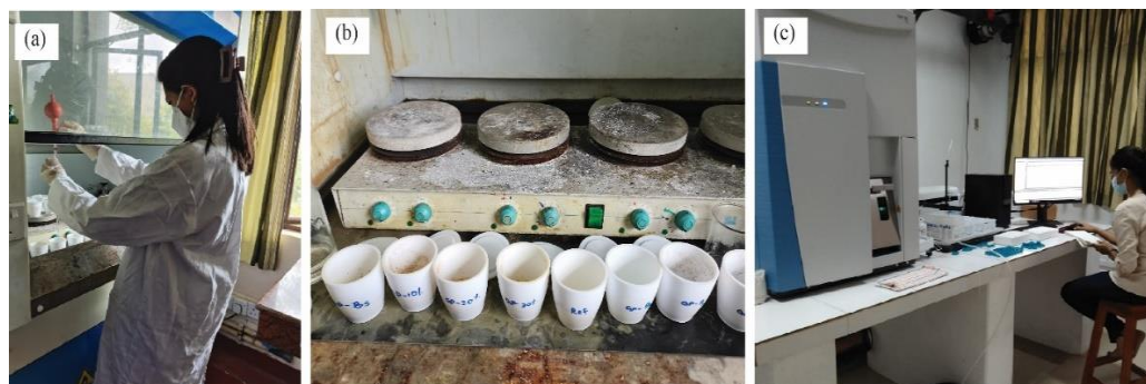
Figure 3. 6 (a) Soil sample digestion with HNO 3 , HCl, and H 2 O 2 ; (b) Digested soil samples; (c) Sample analysis for Ni, Cr, and Co in serpentine soil and rock.
