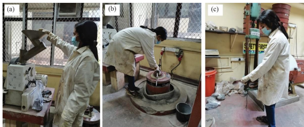
Figure 3. 5 (a) Crushing serpentinite rocks to reduce the particle size using laboratory jaw crusher; (b) Powdering rock/soil using laboratory Tema mill; (c) Sieving through 63 \mu\text{m} sieve to reduce the particle size.
