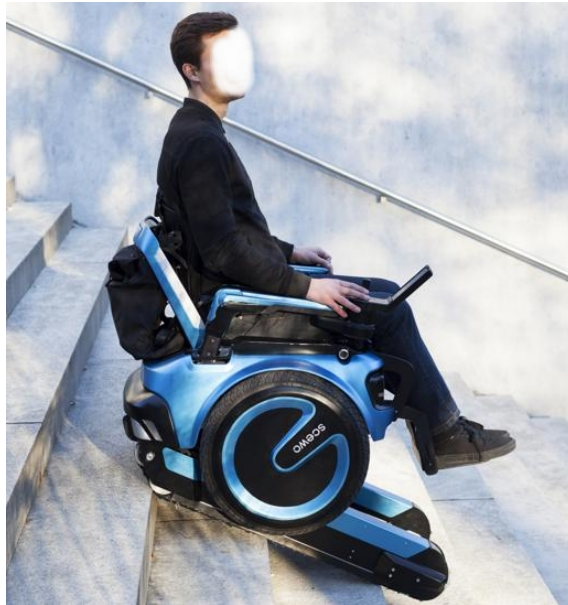
Figure 2.6: Track based stair-climbing wheelchair operation on a staircase
