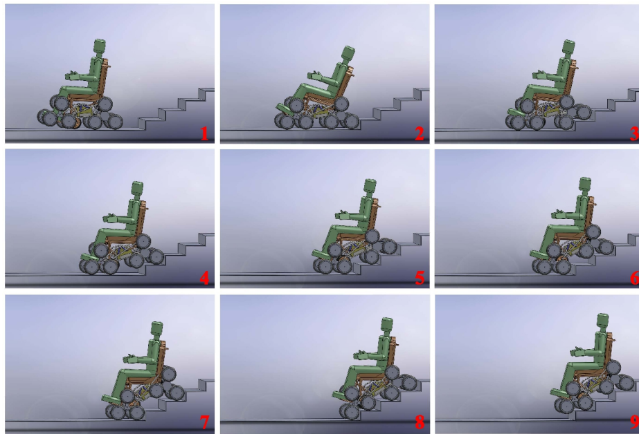
Figure 2.4: User placement oscillation in wheel based mechanism
