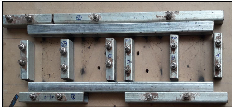
Figure 3.8: Mould of side frame for bearing placement
