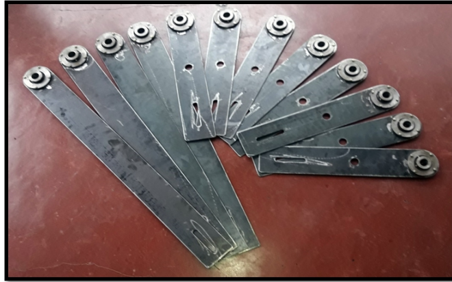
Figure 3.13: Constructed arm plates in prototype
