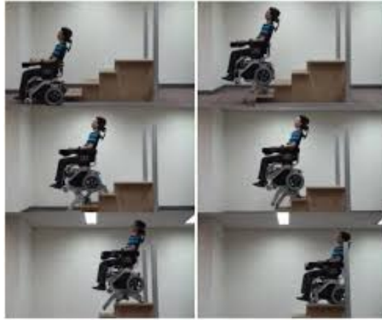
Figure 2.5: User placement oscillation in leg based mechanism
