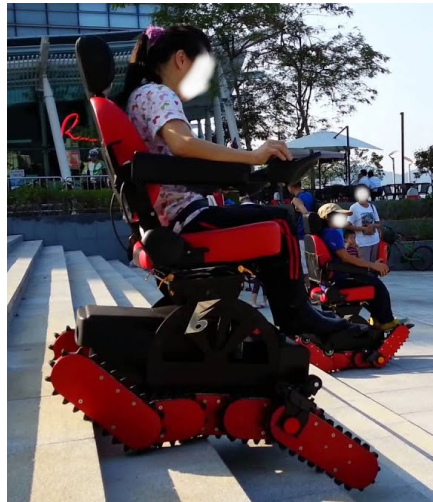
Figure 2.9: B-Free wheelchair operation over a staircase
