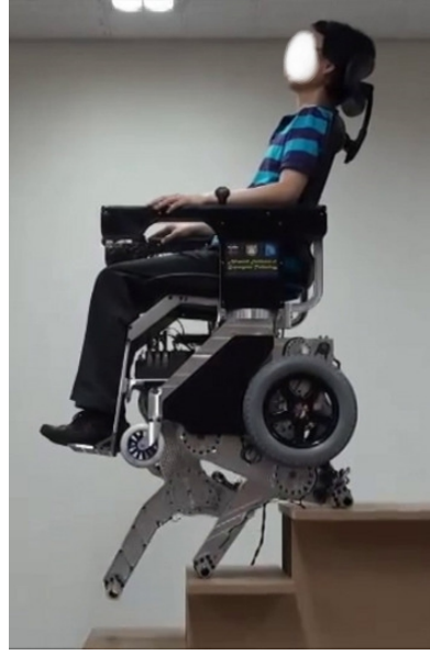
Figure 2.2: Leg based stair-climbing operation
