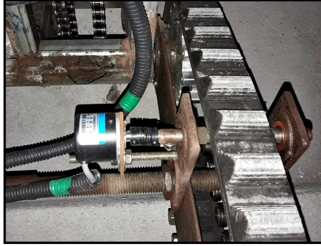
Figure 4.4: Incremental rotary encoder placement on arm
