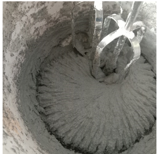
Figure 9: Mechanical mixing of the control mix using a hand-held mechanical stirrer.
