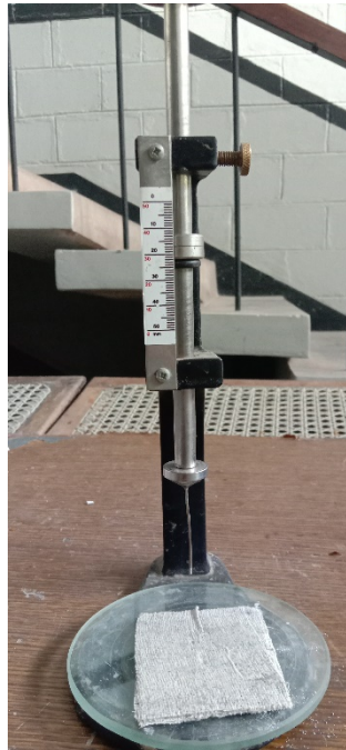
Figure 41: Vicat apparatus set up for initial and final setting time measurement of the tested samples
