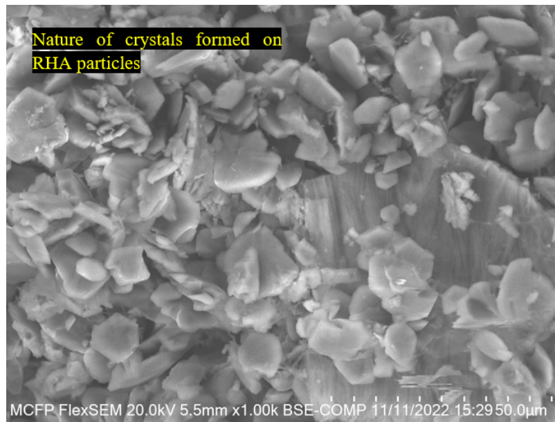
Figure 33: Crystal formation in 15% RHA modified samples x1000
