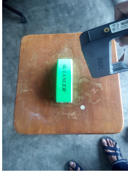
Figure 3.2: Manual Scanning using Portable 3D Scanner
