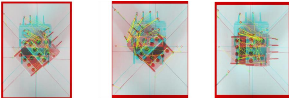
Figure 5.10: Object 01(Contactor relay plastic cover) surface feature extraction in different angular positions
