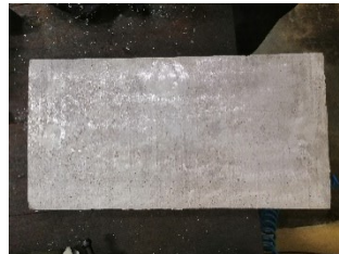
Figure 5-7: Aluminium plates 450mm x 250 mm x 30mm
