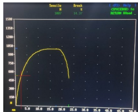
Figure 4-4: Force Vs. Elongation graph for tensile test
