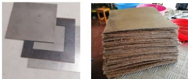
Figure 5-1: Mild steel mold with cover plates and prepared composite sheets
