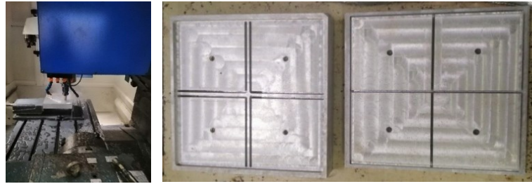
Figure 5-9: Casting work process of the mold and male and female molds
