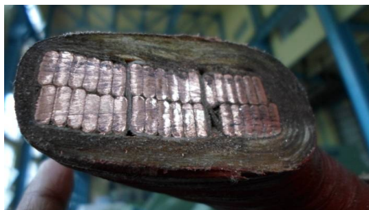
Figure 1:3 Physical cross section of winding
