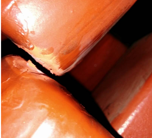
Figure 5:19 PD Symptoms observed from GT 07 on 2014.08.13
