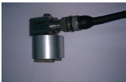
Figure 4:4 SKF CMSS2200- Data acquisition equipment and structural layout
