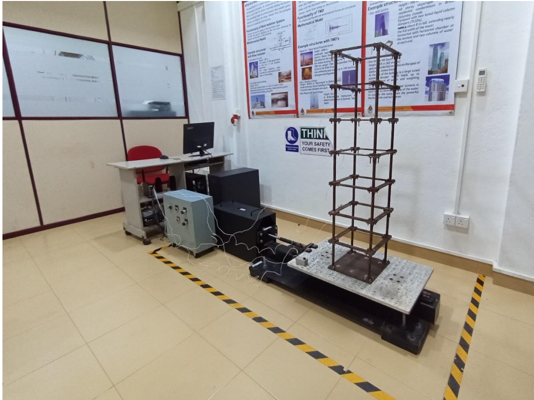
Fig. 3.2: Shake table test setup and steel framed structure mounted on top of the shake table
