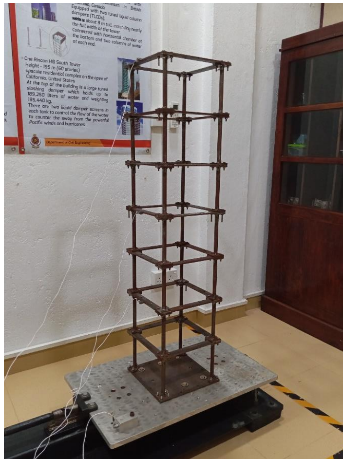
Fig. 3.5: Undamaged structure prepared for the experiment on top of the shake table
