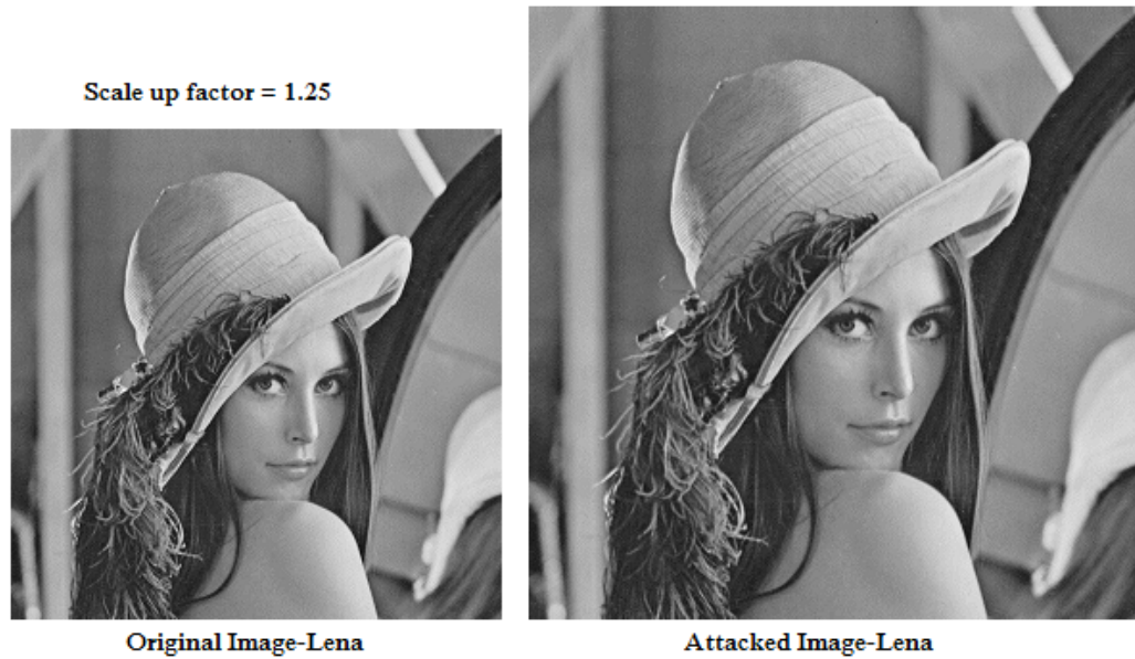
Figure 3.6: Image Resize Attack on Lena Image:ScaleUp
