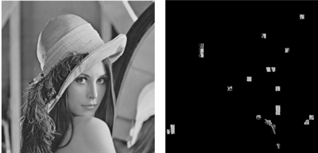
Figure 2.23: Hybrid watermarked still image “Lena” with 18 bits embedded (left), difference to original (right)
