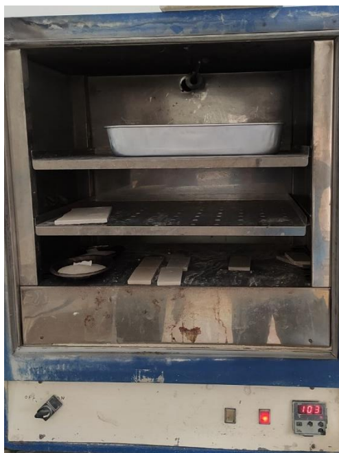
Figure 3.3 Drying PALP by laboratory drier
