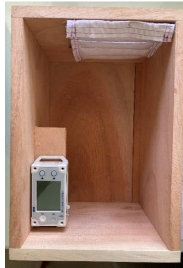
Fig.2- Top view of the PCM insert curtain applied Chamber
