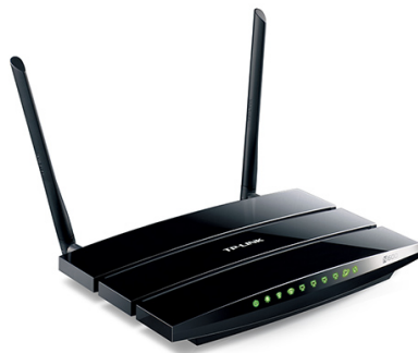
Fig. 2.29: TL-WDR3600 Router containing a Atheros NIC [18]
