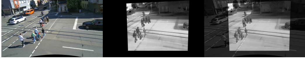
Fig. 2.10: Visualization of Pedestrian crossing data in R-LiViT with left being original, middle being thermal image and the right being both image overlaid [6]
