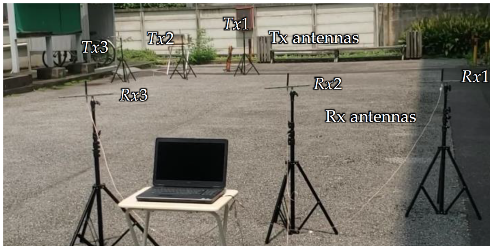
Fig. 2.20: Actual setup of [11] using 3x3 MIMO links to the Wi-Fi device connected to the Laptop
