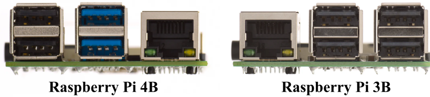
Fig. 2.33: USB-Ports of Raspberry Pi 4B vs 3B
