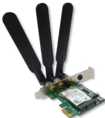
Fig. 2.28: Intel 5300 NIC with its extended 3-Antenna setup using an adapter [17]
