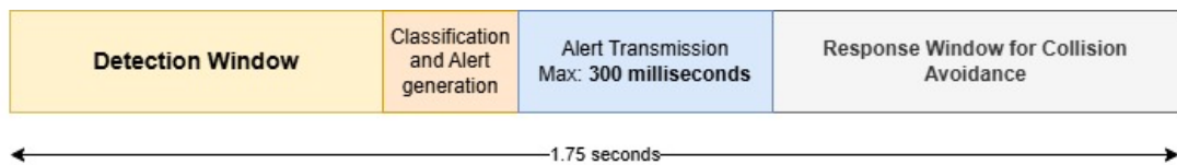
Fig. 2.38: Illustrated End-to-End Time Window for VRU applications defined by ETSI
