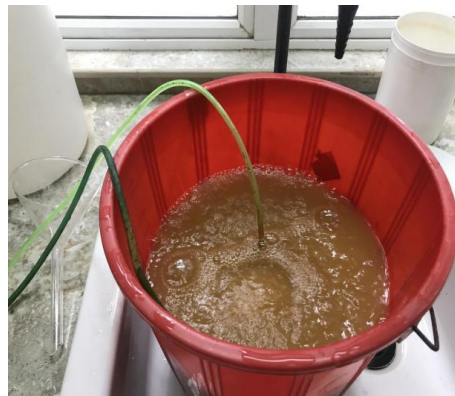
Figure 3. 11: Aerating the wastewater with Fenton reagent
