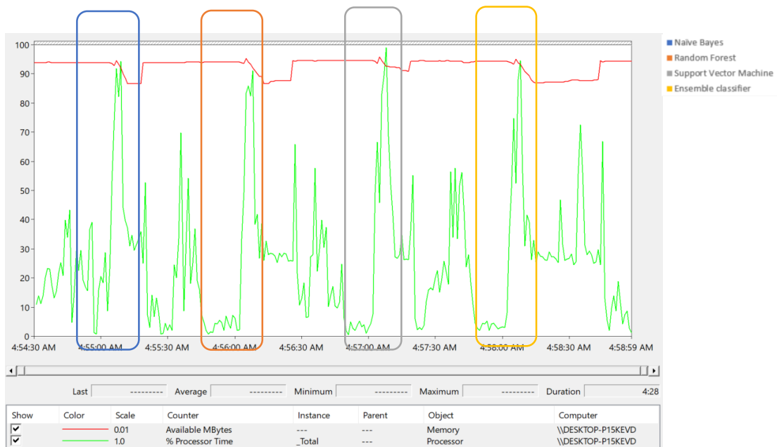
Figure 5.2.2: Server resource usage by training process by each classifier – Root Node
