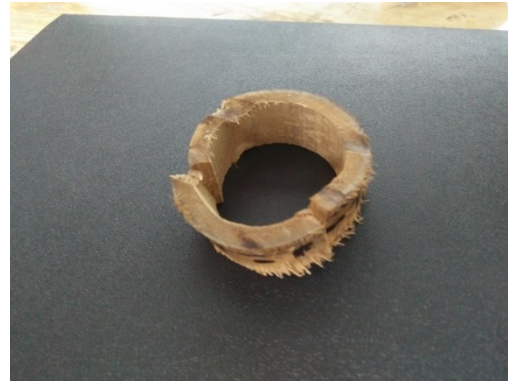
Figure 4.12: Failure pattern 58-T-Top sample in flat ring flexure test
