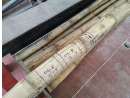
Figure 3.15: Samples being marked on a pole prior to cutting
