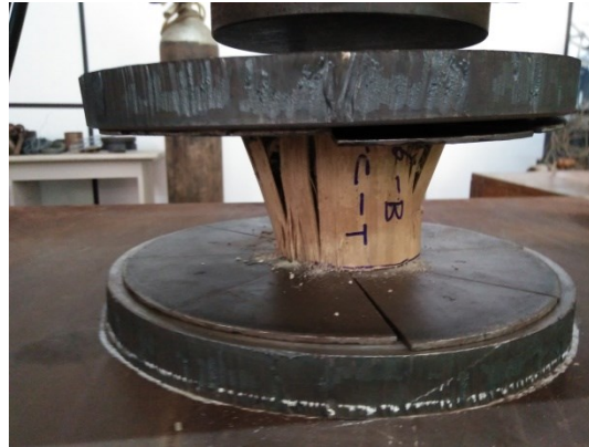
Figure 4.2: Failure of 06-B-Top during compression loading
