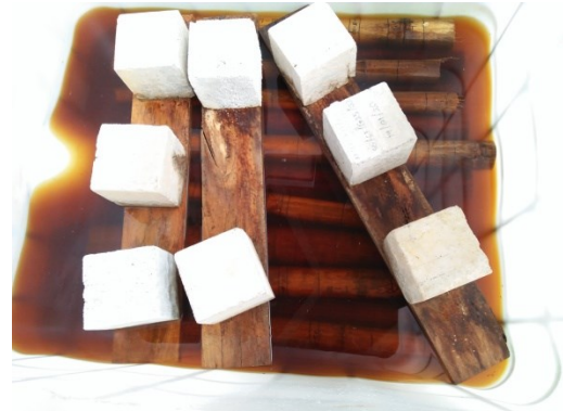
Figure 3.14: Preservation treatment of poles (day 7)
