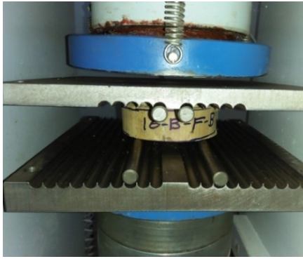
Figure 3.19: Flat ring flexure testing with standard compression machine
