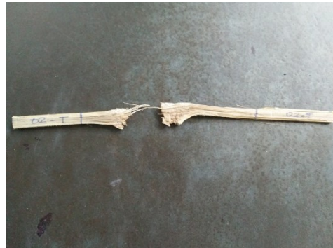
Figure 4.16: Tensile failure at node of 02-B-Top sample
