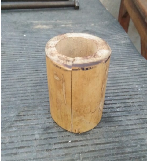
Figure 4.7: Shear failure pattern of 58-T-Bottom sample
