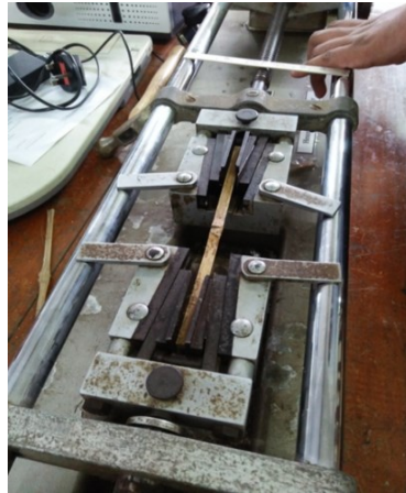
Figure 3.21: Tensile testing with Hounsfield Tensometer
