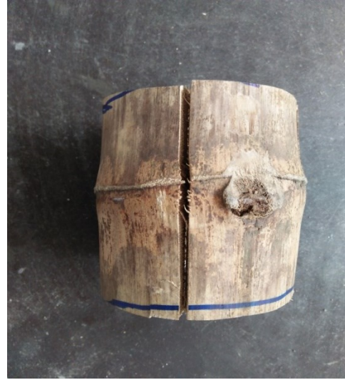
Figure 4.8: Shear failure pattern of 07-B-Bottom sample
