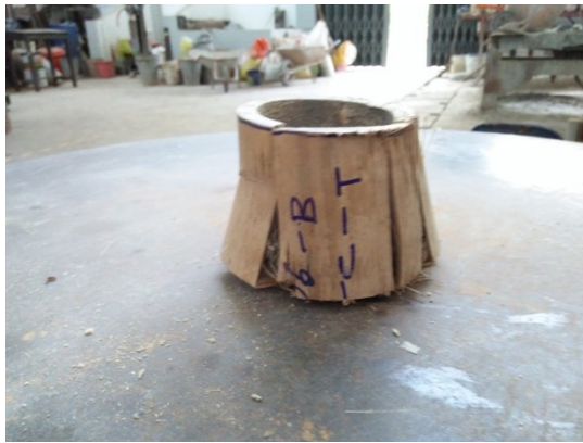
Figure 4.3: Compressive failure pattern of 06-B-Top
