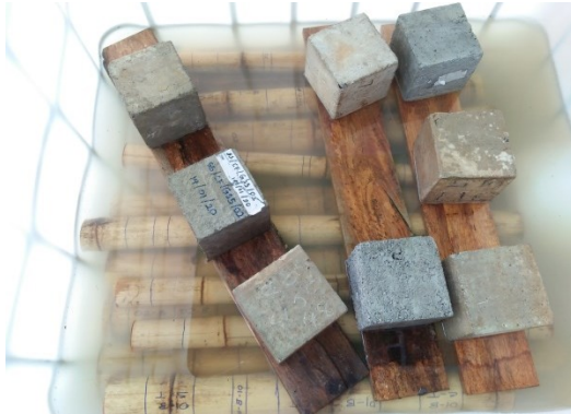
Figure 3.13: Preservation treatment of poles (day 1)
