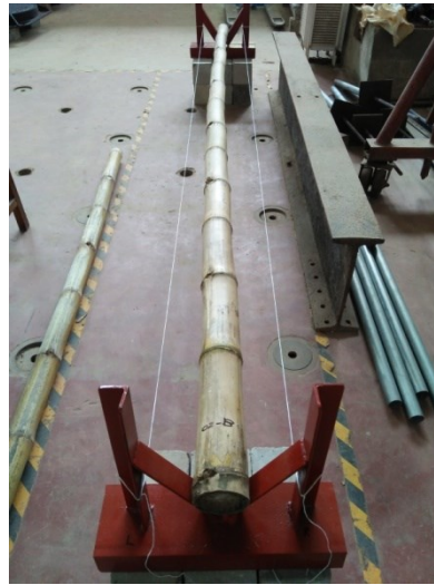
Figure 3.10: Data measurement setup for a bamboo culm
