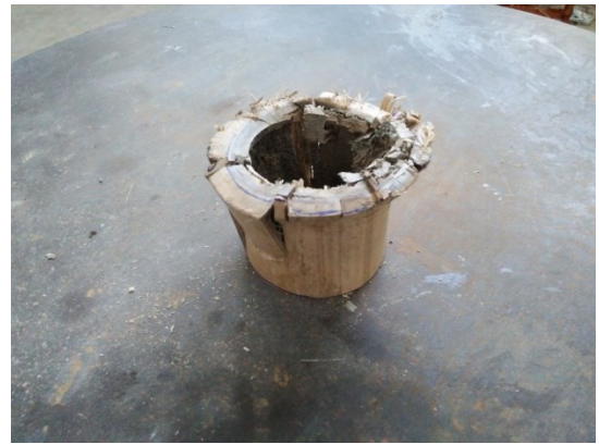
Figure 4.4: Top view of compressive failure pattern of 06-B-Top
