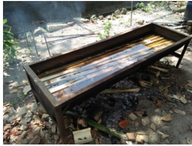
Figure 2.9: Treatment in trough
