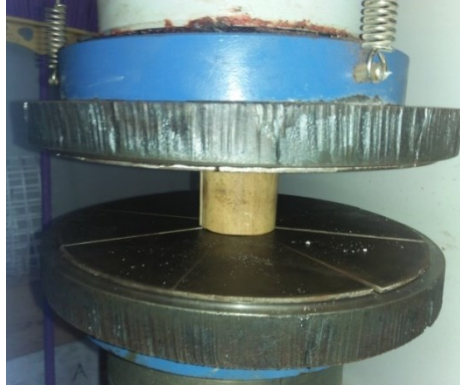
Figure 3.17: Compressive strength testing with standard compression machine
