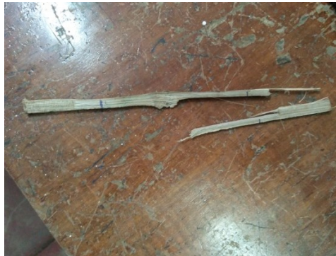
Figure 4.15: Tensile failure between grip and node of 58-T-Top sample
