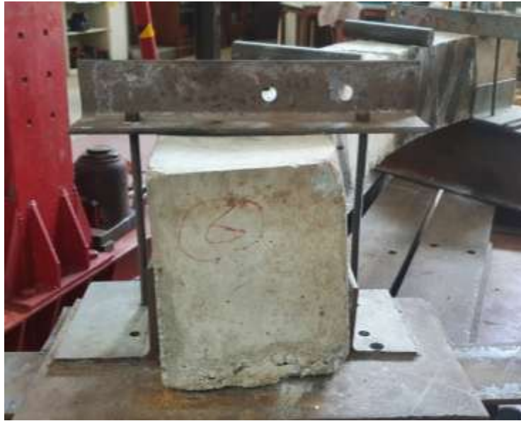
Figure 19: End clamp to prevent rotation and twisting
