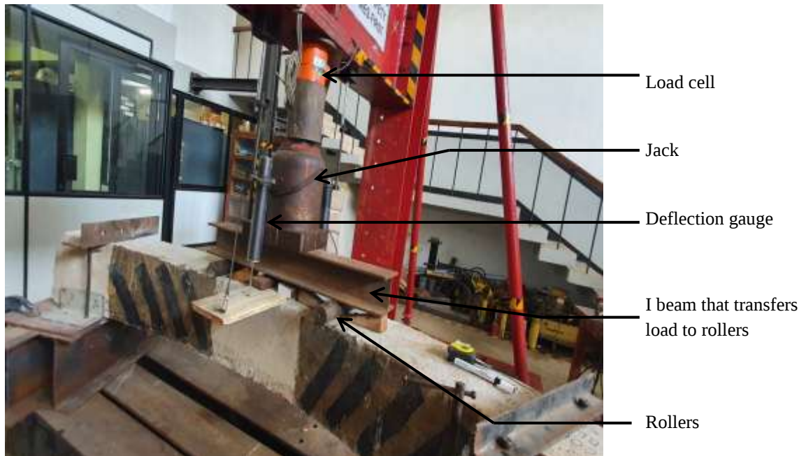
Figure 20: Load points and loading method
