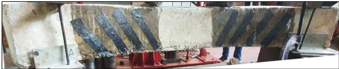
Figure 16: Shear retrofitted beam
