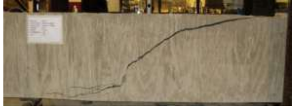
Figure 5: Shear failure modes and crack patterns (a) diagonal tensile failure with shear links (b) diagonal compressive failure (c) diagonal tensile failure without shear links (Dinh et al., 2011)
