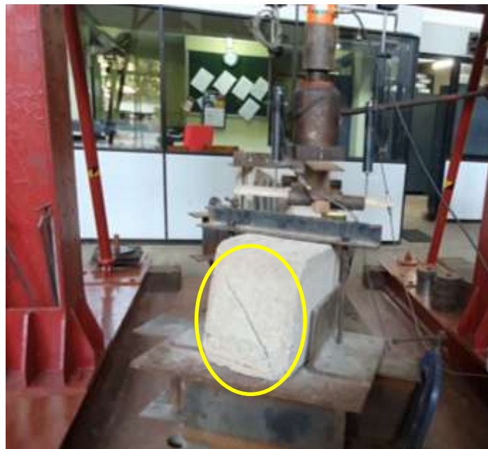
Figure 33: Torsional crack at beam end – Beam C
