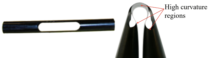
Fig. 1.5 A composite tape-spring hinge subjected to high curvatures.
