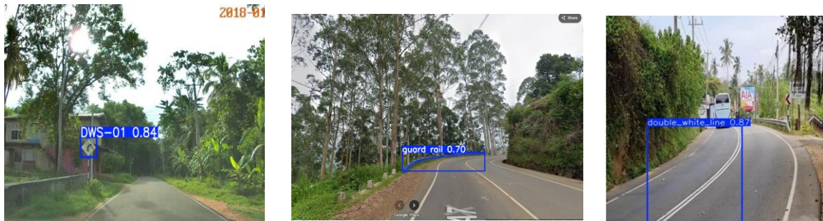
Figure 7. Detection results: road sign DWS-01 (left), guardrail on A7 (centre), double white line (right)
