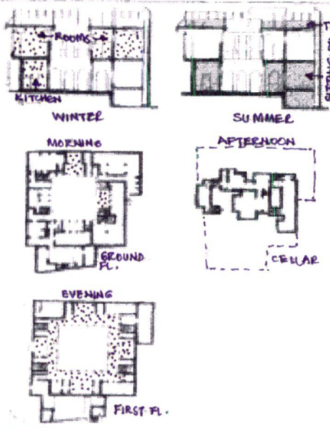
Fig.7 - The rooms are distributed round the courtyard so as to allow them to be used for different purposes, depending on the time of the day or the season of the year, these particular drawings are of a house in Baghdad. (Source: The history of the city, Benevolo)
