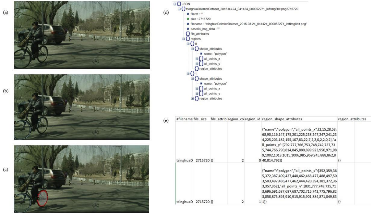
Figure 3.3: Wheel annotation with VIA. (a) Original image; (b) Annotation of front wheel; (c) Annotation of rear wheel; (d) JASON file of annotations; (e) CSV file of annotations
