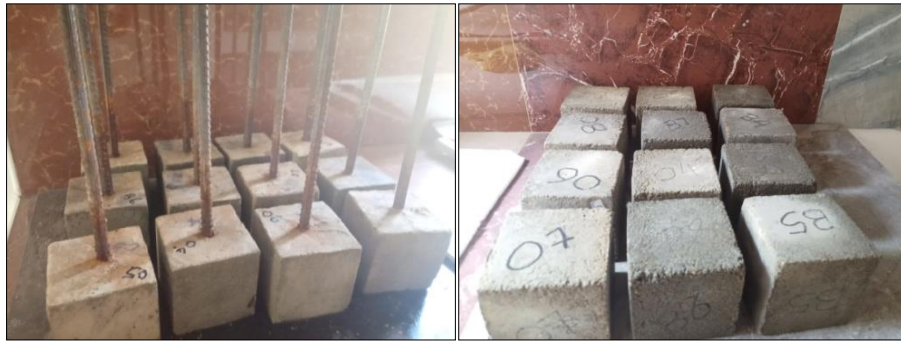
Figure 3.1.4: Test specimens for salt conditioning
