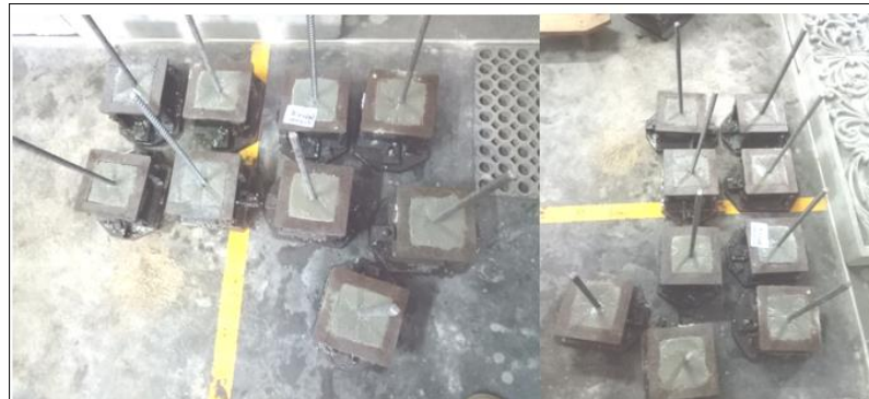
Figure 3.1.1: OPC and PPC specimens (for pull out test), after casting
