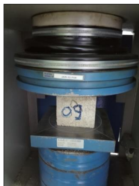
Figure 3.2.1: Compression testing of cement motor cubes
