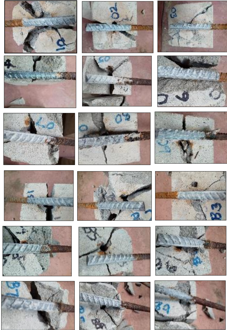
Figure 4.4.2: TMT steel bars after pull out test
