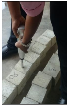
Figure 3.1.7: Testing with Rebound Hammer instrument
