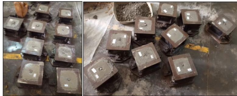
Figure 3.1.2: OPC and PPC specimens (for compression test), after casting
