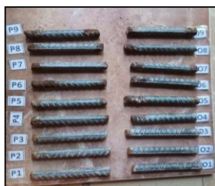
Figure 4.5.2: Ribbed Steel bars after separating from the cubes
