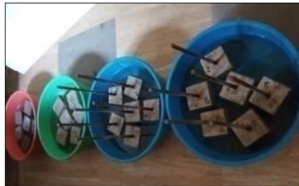
Figure 3.1.5: Test specimen in salt baths
